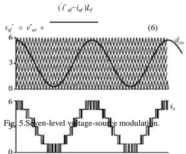
Fig 5. Seven-level voltage-source modulation.
