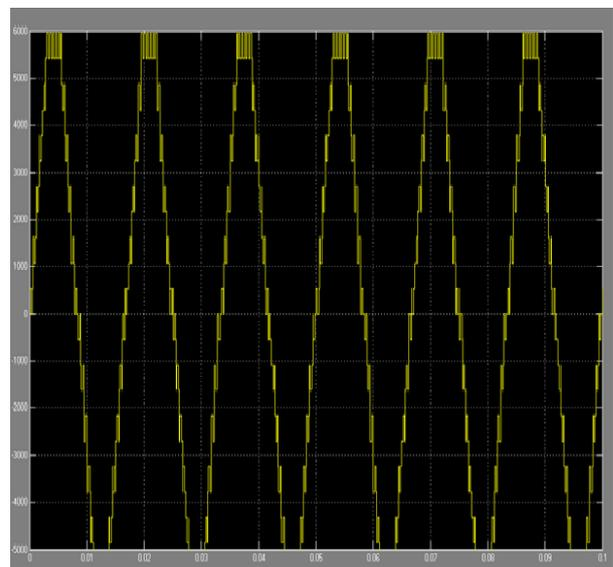
**Fig :Reactor terminal output Voltage Waveform**
