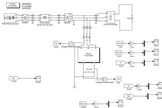
**Fig: Seven-level Shunt Active filter Simulation Diagram**
